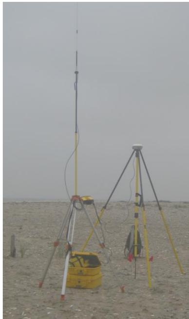
Base station configuration (left: external radio; right: R8 base receiver). Photo: M. Weakley, 2010.
