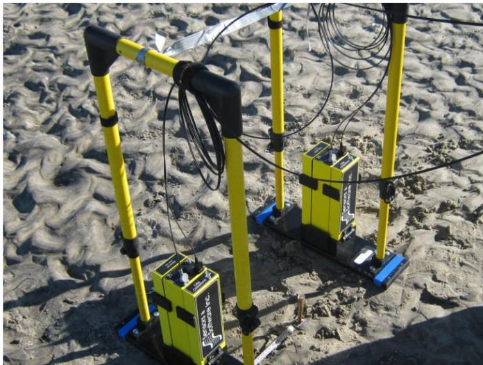
Stepwise GPR configuration, with antennae (transmitter and receiver) resting on the ground surface. Photo: D. Oster, 2010.
