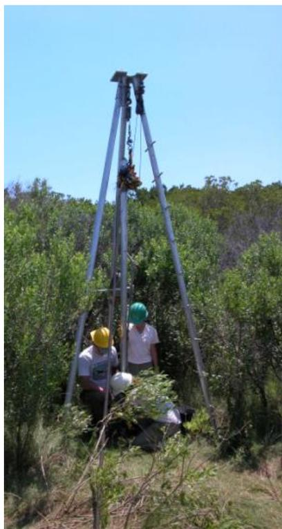
The vibracoring rig on Hog Island, showing tripod, core pipe, and concrete vibrator attached to top of core pipe (engine not shown). Photo: R. McBride, 2010.
