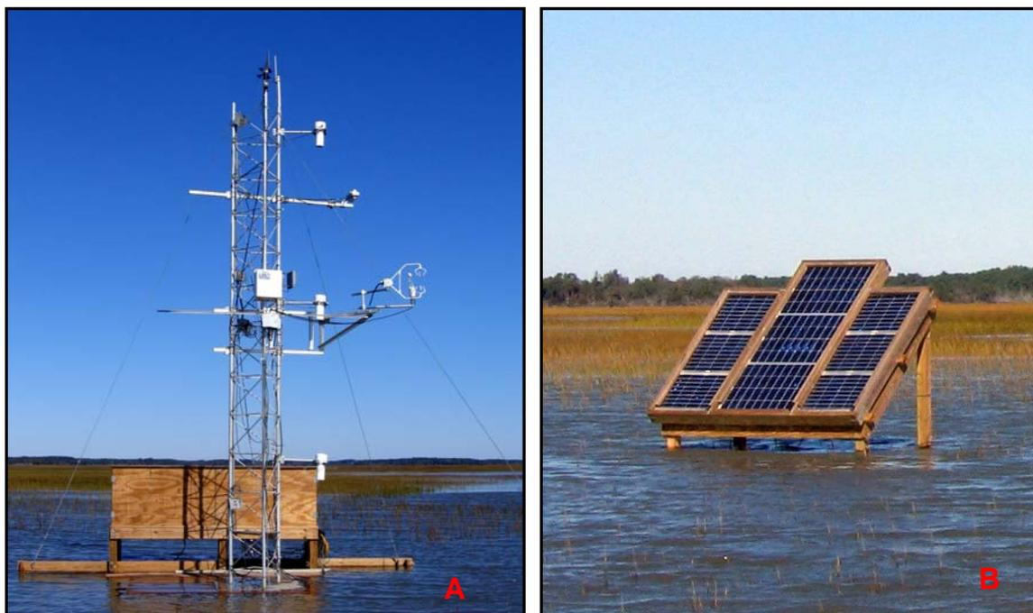
Figure 1.4. A) Flux tower set up with instrumentation along with the battery bank platform during high tide conditions, and B) solar panel setup showing the nine panels framed and mounted above the sediment.
