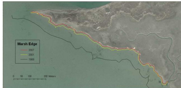
Fig. 12. An ArcGIS image depicting the marsh edge at Chimney Pole marsh in 1968, 2001, and 2007 based on aerial photos. The edge at Chimney Pole has been eroding about 1.57 m/yr from 1968 to 2007 and about 1.21 m/yr
