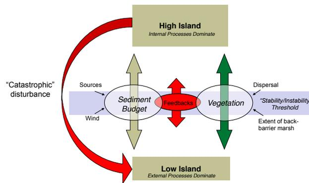
**Fig. 20.** Ecogeomorphic framework for barrier island evolution, showing feedbacks between vegetation and sediment supply, which over time result in the development of two large-scale morphologies with either high-relief, less frequently disturbed islands or low-relief overwash-dominated islands.
