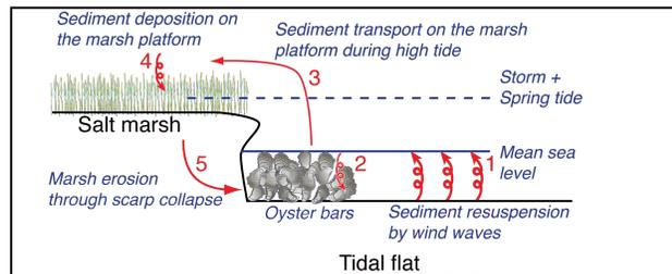
**Fig. 24.** Oyster bars adjacent to intertidal marshes may reduce the sediment supply and wave energy hitting the marsh boundary, and influence state change dynamics. Arrows represent sediment fluxes: 1) resuspension, 2) sedimentation, 3) transport to marsh platform, 4) deposition, and 5) marsh edge erosion.
