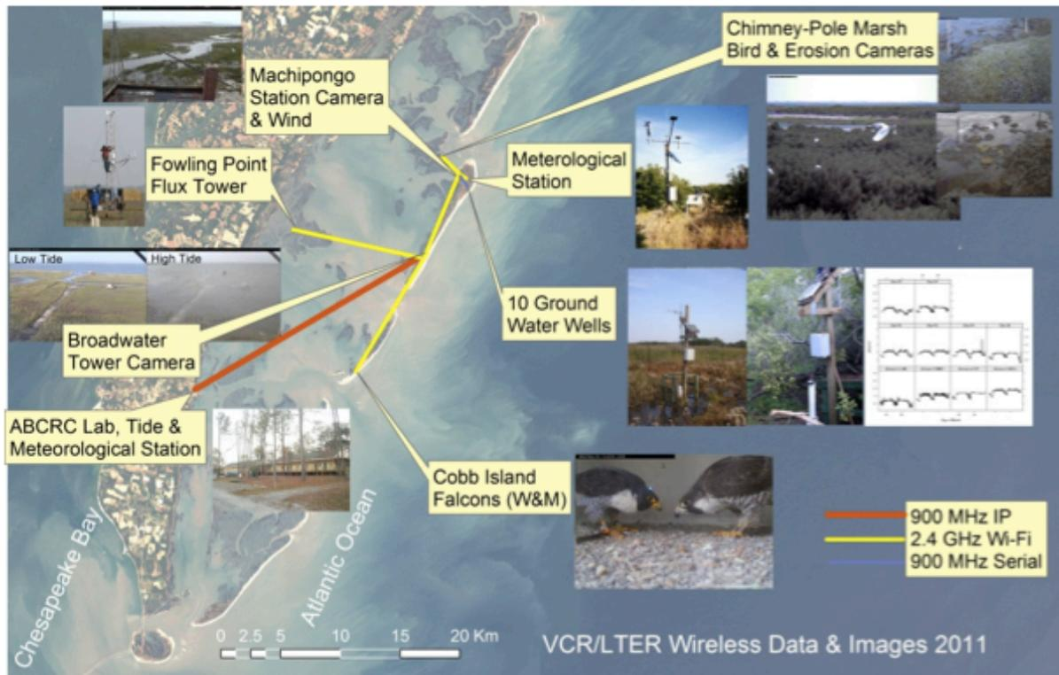
**Fig. 3.** The VCR/LTER Wireless Network extends from the ABCRC laboratory to our main island research areas and connects a wide variety of instrumentation, including data loggers and cameras. Workflows are used to automate processing of data to provide near real-time online access.
