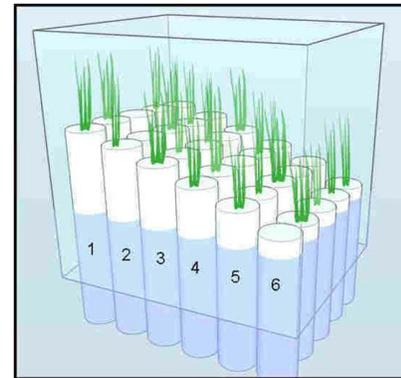
**Fig. 21.** The white cylinders are submerged at different depths in the water. The plants submerged deepest (row 6) experience the highest sea levels. The plants elevated highest (row 1) experience the lowest sea levels. (Credit: Adam Langley/SERC).
