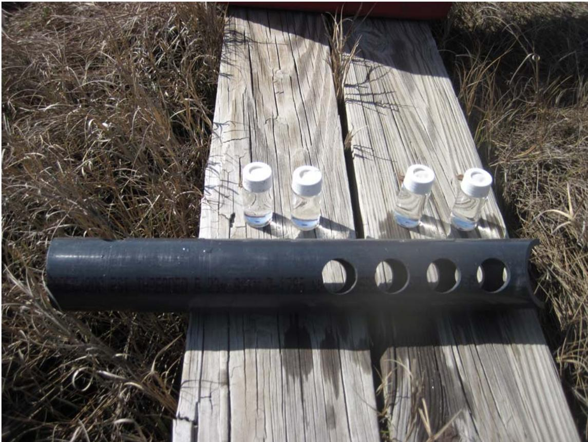
Figure 3. Photograph of PVC equilibrator alongside capped vials. The vials were inserted into the holes in the PVC pipe, which was then placed in the ground to equilibrate for four weeks.
