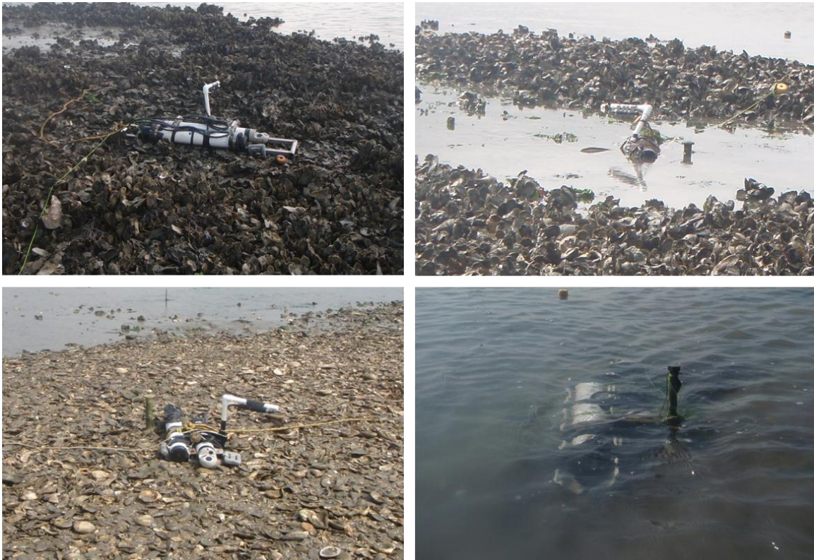
Figure 2.14: The four AQDPs deployed for the Multi-site study; (A) HLCR2, the historical reef; (B) HLCR WHELK, the whelk shell restoration site; (C) HLCR 2008, the fossil shell restoration site; and (D) HLCR MUD, the mud site between HLCR2 and HLCR WHELK; Note: In A, B, and C OBS are deployed with the AQDPs on PVC arms.
