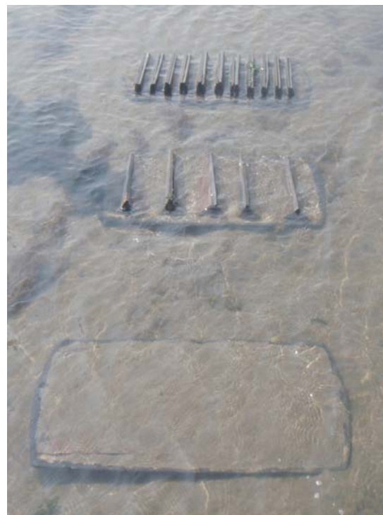
Fig. F24. Structure manipulation experiments showing three different geometries of slate plates. Note the large sedimentation and no visible recruitment on the tray with flat plates.
