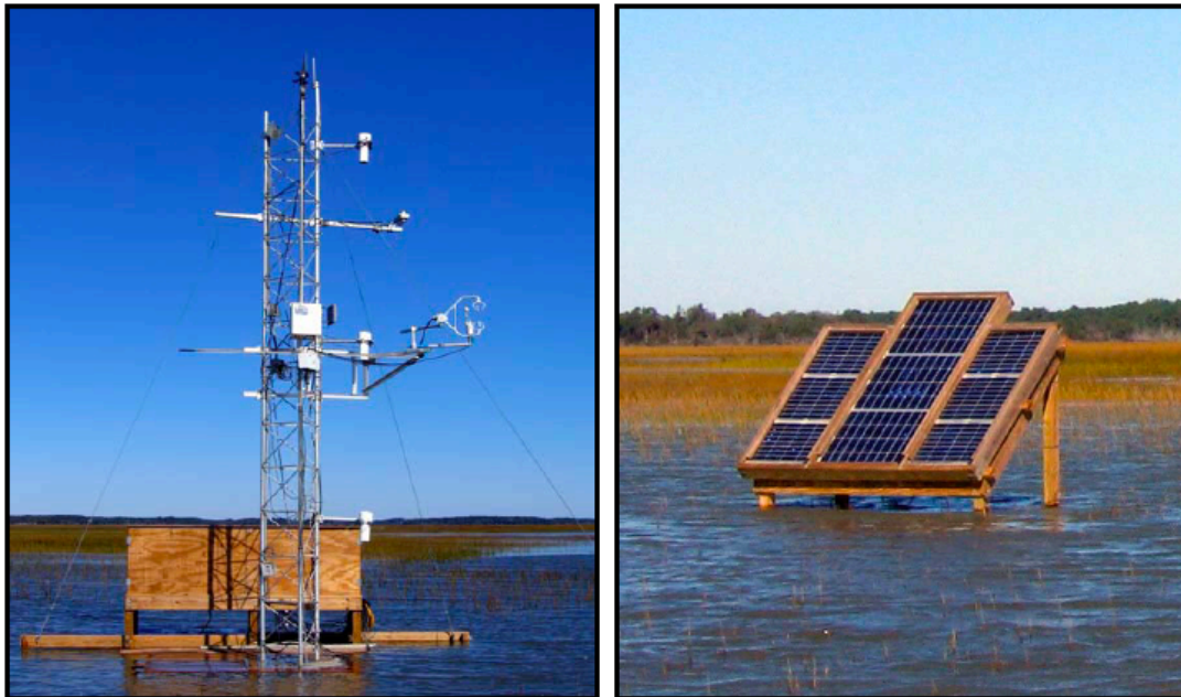
Fig. 6. Flux tower (6.7m) on Fowling point marsh at high, with solar panels that power instruments.
