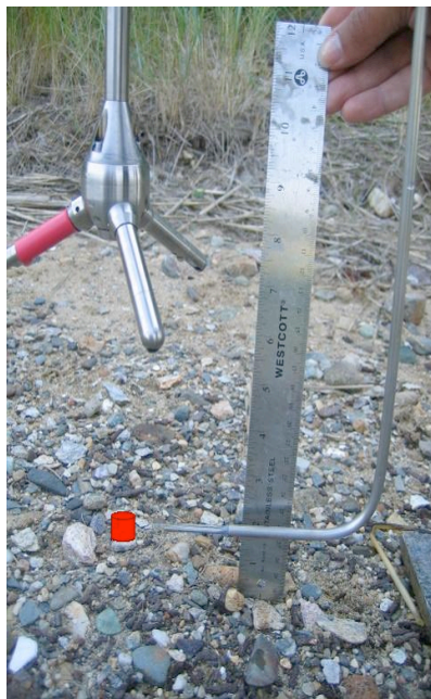
Fig. 3 (left). The eddy correlation system for measuring groundwater fluxes from the sediment to the overlying water consists of an Acoustic Doppler Velocimeter (ADV) and a fast conductivity and temperature sensor (PME). Fig. 4 (right). The groundwater flux can be determined by the heat flux over a 5-m long footprint.
